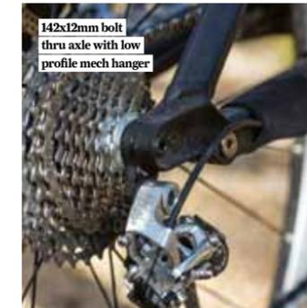
142x12mm bolt thru axle with low profile mech hanger
